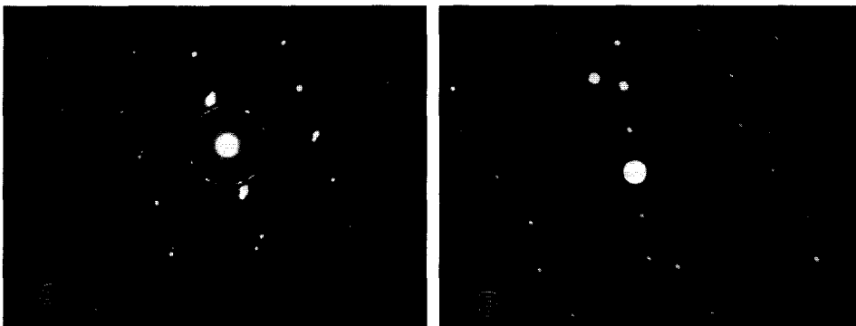
Fig. 3. Selected area diffraction patterns for two orientations of the \alpha'' plates shown in Fig. 2.
