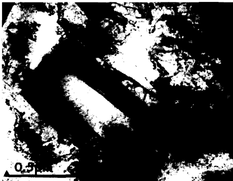
Fig. 2. TEM micrograph showing martensitic plates formed in quenched U–3.6 at.% Ti–4.7 at.% W alloy. The plates were identified as \alpha'' monoclinic phase.
